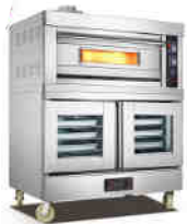
Baking with Proofer, Gas 1 Deck 2 Tray Model: EFC-102QF, Ecoline, Sinmag, Salva Size (mm): 1340x900x1620, Weight: 465kg Power: 2.8Kw/ 220V
