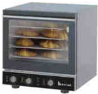
BUTLER Convection Oven with Steam Model: ECO-004S, Cap.: 4 Trays Size: 760x840x790 Power: 230V, 5.8kW, 44Kg
